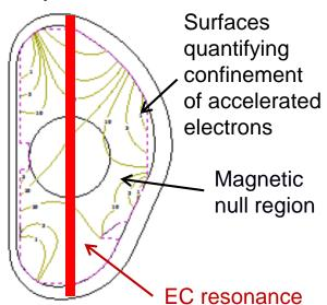
EC will assist plasma initiation to ensure robust start-up for a wider range of plasma conditions.
